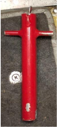
Be-76 Gear Tool and its stowage in the cockpit. Access to the operation mechanism is under a flap at floor level. Operating instructions are also provided.
